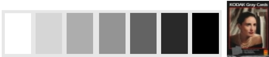
Fig. 4. Comparison with gray cards is used to determine the gray scale of an unknown tone. Left: gray cards (see web site); right: a gray card book (see web site).
