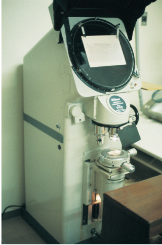
Fig. 4-2. A profile microprojector, Nikon model V-16C, useful for picking up necessary contours of structure from serial sections at various magnification.
