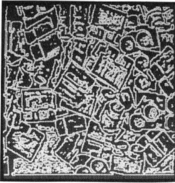
Fig.3c Edge map. The edge map is obtained by differentiating the brightness distribution.
