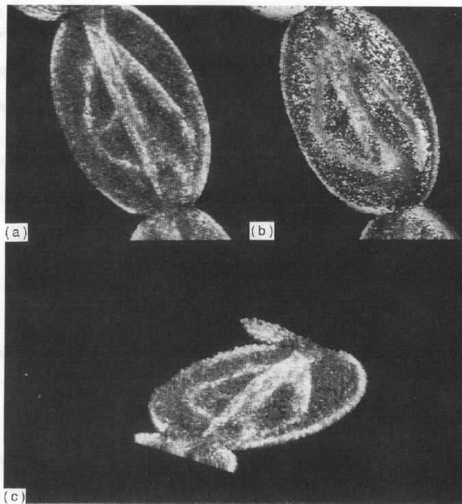
Fig. 13. Tradescantia stamen hair cell. (a) autofocus image created in the same way as the left half of the stereo pair in Fig. 12. (b) surface profile image where a grey scale has been used to code the significant bits in the image according to their location in depth (light grey=top, dark grey=bottom of cell). (c) isometric projection using information from both (a) and (b).
