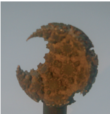
Fig. 3. Copper model of 3D quasi-Fuchsian fractal with inkjet based 3D printer and lost wax investment casting.
