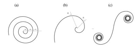
Fig. 1. Three basic spirals. (a) The Archimedean, (b) the logarithmic and (c) the Comu's spirals.
