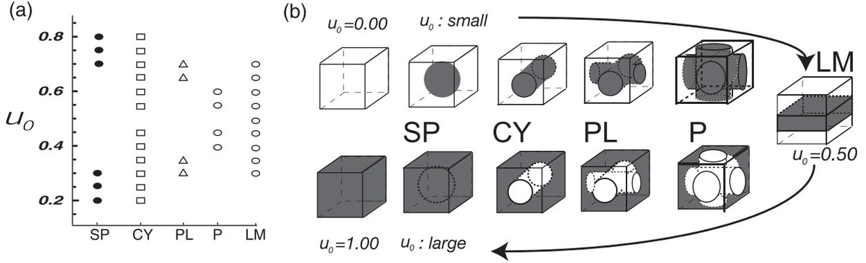
Fig. 1. (a) Five stationary solutions for  $D_u = 1.0$ ,  $D_c = 50.0$ ,  $\beta = 10.0$ ,  $k^2 = 50.0$ , and  $\lambda = 40.0$ . The explanations of SP, CY, PL, P and LM are provided in the text. (b) Schematically showing the obtained patterns SP, CY, PL, P and LM.
