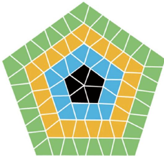
Fig. 4. The most fundamental concentric tiling of regular pentagons is generated by arranging five “golden trapeziums” ( 108^\circ - 108^\circ - 72^\circ - 72^\circ ) dextrally around a vertex in the central area and the pattern is concentrically inflated by adding more tiles around it as shown.
