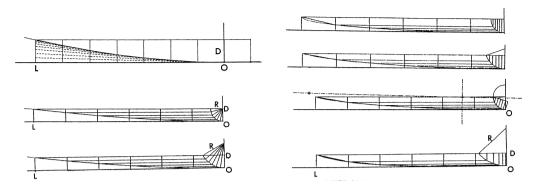
Fig. 4. Various Drawing Procedures for Curves of Eaves.
