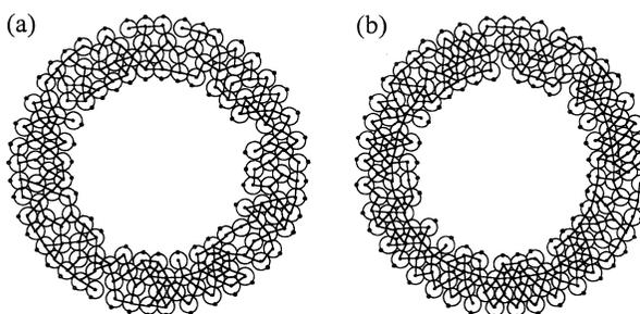
Fig. 3. Disk contact networks: a) the disk contact network obtained at the experiment of packing fraction 0.74, b) one of 0.76.
