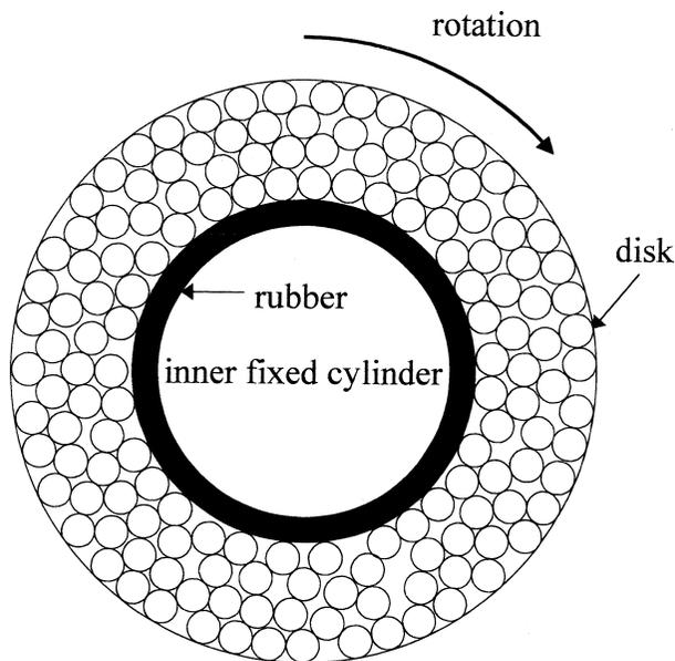
Fig. 1. Experimental setup. An annular cell consists of the outer rotating cylinder and inner fixed cylinder.
