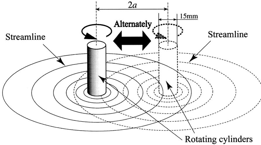
Fig. 1. Schematic illustration of two-dimensional flow model.
