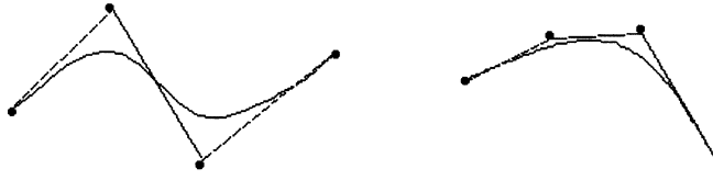
Fig. 4. Deriving B-spline curve control points and control polygon for strokes.
