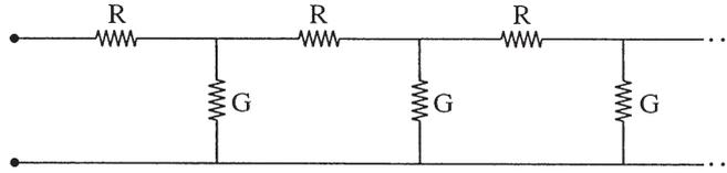
Fig. 6. An infinite ladder circuit with resistances  $R$  and  $G$ .
