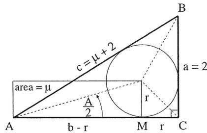
Fig. 5. The geometry of a right triangle represents the trajectory values  $p$  and  $q$  after a period doubling bifurcation where the radius of the inscribed circle  $r = -q$ , line segment  $AM = p$ , and the area of the rectangle formed by  $r$  and  $AM$  equals  $\mu$ .
