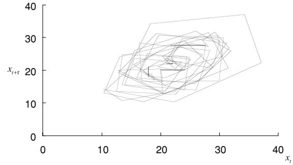
Fig. 4. An example of the attractor reconstructed from the EGG time-series data (100 sec.).
