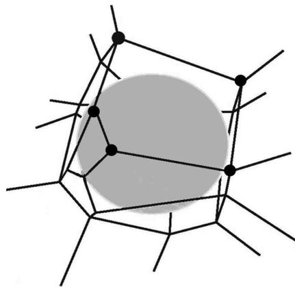
Fig. 10. Shape of polyhedral cells are described by vertex positions.
