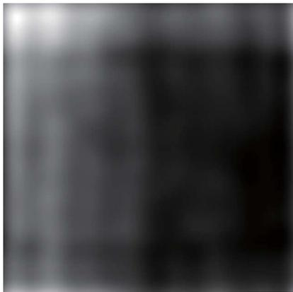
Fig. 6. The stationary noise image. An X-ray image processed using an LPF (cutoff frequency: 0.195 cycles/mm).
