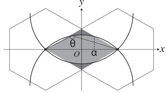
Fig. 4. Region such that  $\Theta \leq \theta$  for the triangular lattice.
