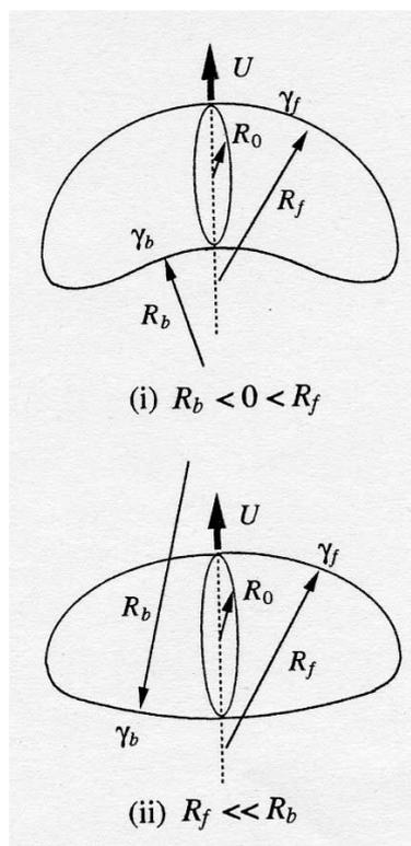
Fig. 3. Illustrative figures of the equilibrium shape of a drop under non-uniform distribution of surface tension.
