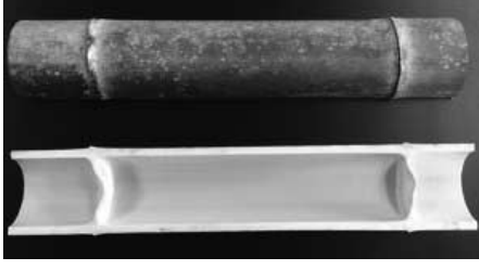
Fig. 2. Cross section of a bamboo culm segment. Reprinted from Ref. [7] with permission.
