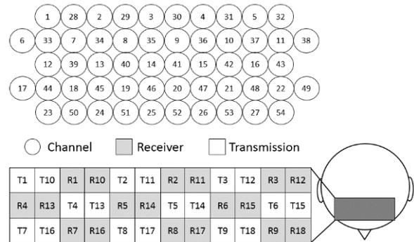
Fig. 3. Array of irradiation and light-receiving probes.
